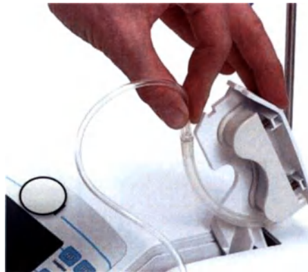
Pic 6. To access the pump, press release key by the display on the front of the control unit. It can be easily done with one hand, without inadvertent moving of the device
