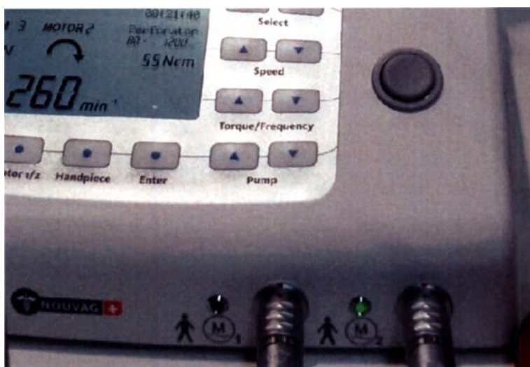
Pic. 2. Two 21 electric motor sockets on the control unit.
