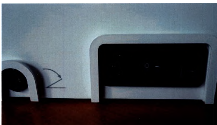
Pic. 3. Pedal socket on the rear panel of the control unit.
