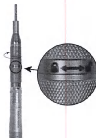
Figure 47: Turning the Tool Lock to the Locked Position
