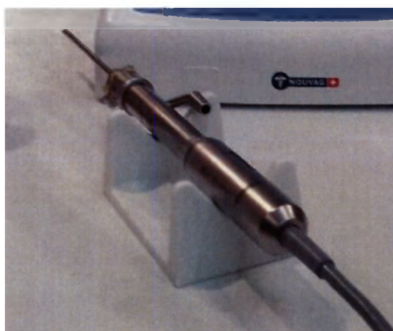
Picture 21. The handpiece attached to the electronic motor resting on the handpiece cradle.
