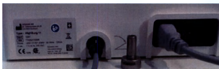
Pic. 20. Device with plugged in the electric supply and pedal cables
