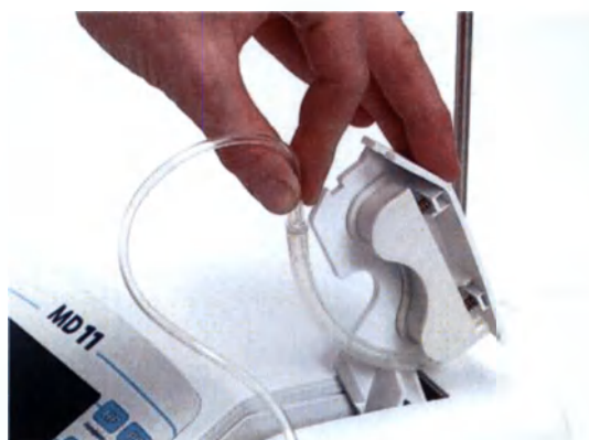
Picture 14. To access the pump, press release key by the display on the front of the control unit. It can be easily done with one hand, without inadvertent moving of the device
