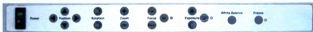
figure 1: the front panel of the Vidi OP system.
