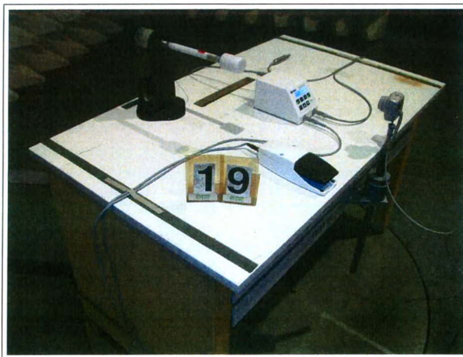
Figure 2 : Test Set-up "Radiated electromagnetic fields and immunity to radiated electromagnetic fields"
