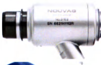
5163 Gear unit with seal unit incl. seals, seal holder and locking wrench (to be assembled as shown in picture 2). The electric motor speed is transmitted through the gear unit to the cutting tube at the appropriate ratio.
