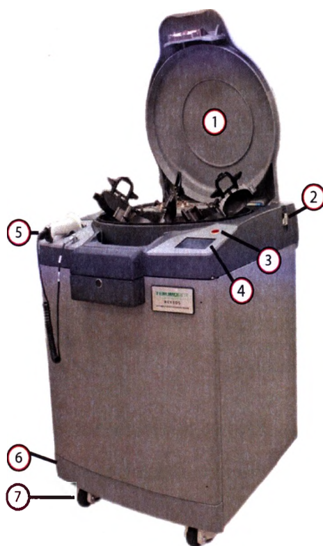
Figure 1: Reveos device with 1) Device lid; 2) Power switch; 3) Stop button; 4) Touch-screen display; 5) Barcode scanner; 6) Access drawer; and 7) Casters.
