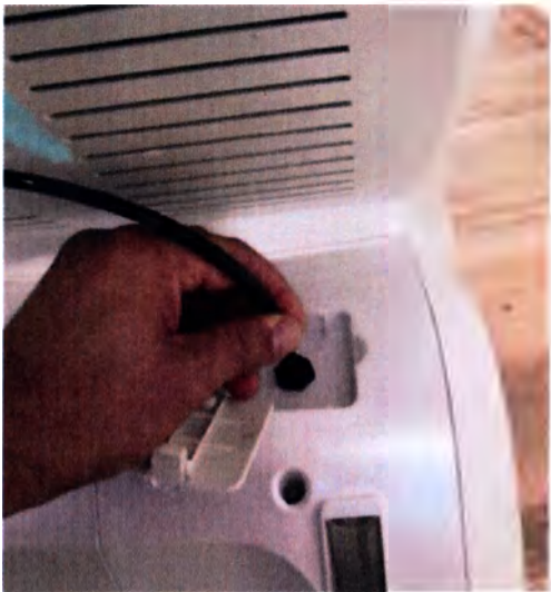
Figure 5.8: Connecting the pipe to the water tank
