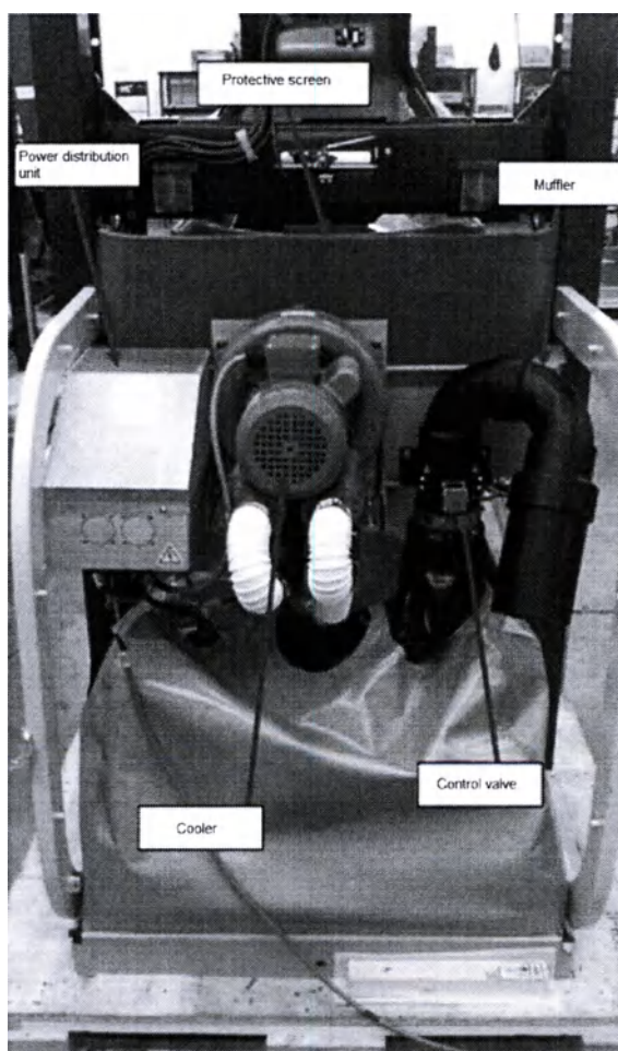
Pic.3: Power unit
