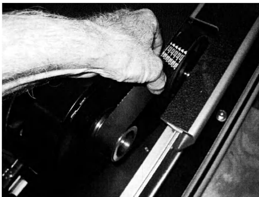
Pic. 31. Checking Drive Belt Tension
