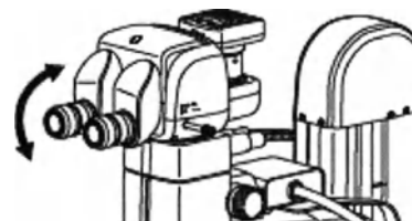
Adjusting the angle of depression
