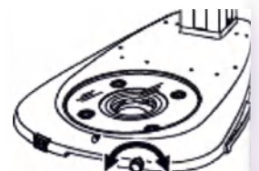
Adjusting the diascopic illumination base
