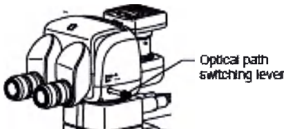
P2-TERG 100/P2-TERG 50 Trinocular Tilting Tube
