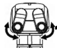
Adjusting the interpupillary distance
