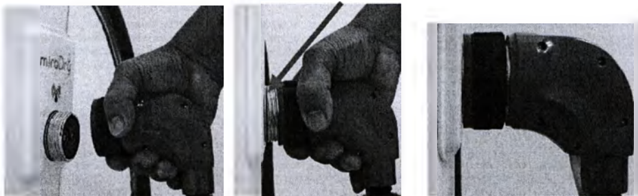
Figure 2 a) Screw on Handpiece b) Red ring still visible c) Proper attachment (red ring covered)
