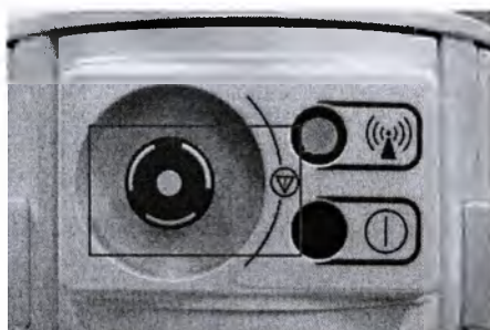
Figure 28: Red Emergency Stop Button
